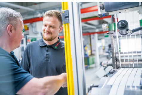
Figure 6 The adhesive tapes are manufactured in-house with no intercontinental supply chains. The high-precision manufacturing processes include laser plotting and rotary die-cutting.
